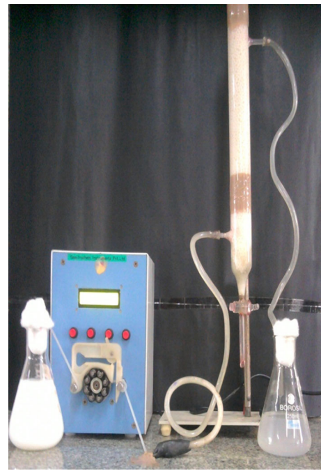
Fig. 2 Reactor packed with Ca-alginate immobilized Ps. aeruginosa
