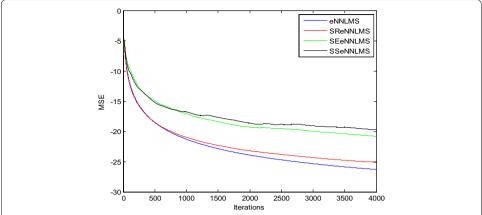
**Fig. 3** Typical convergence curves for ICG signal enhancement in a Gaussian environment using exponential non-negative LMS (eN<sup>2</sup>LMS) and its variants
