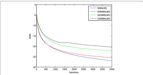
**Fig. 4** Typical convergence curves for ICG signal enhancement in a Gaussian environment using normalized non-negative LMS ( $N^3$ LMS) and its variants
