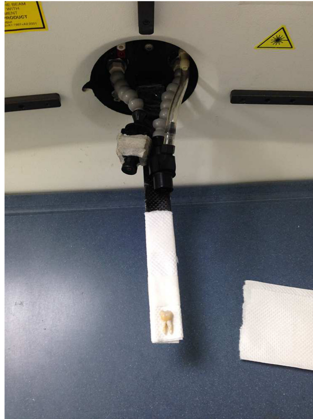
Fig 7. Experimental set-up of MicroCT for tooth scanning.
