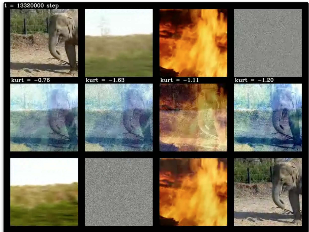
Figure 7. Snapshots of BSS results using movies. Top: Four original images as hidden signal sources. Middle: Four superposed images provided as input to the model. Bottom: The final states of the outputs of the neural network reconstructed the original movies well (Supplementary Movie 2). We retrieved these movies from MotionElements ( https://www.motionelements.com ) and processed them accordingly.
