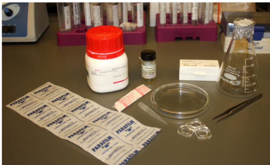
Figure 2. Picture of the common and inexpensive lab materials required for the formation of polymersomes. The items required are: Parafilm, an 18.5 G needle, polymer in chloroform or other appropriate solvent, a 1,000 \mu\text{l} pipette tip, an Erlenmeyer flask, tweezers, agarose, 25 mm square coverslips, PDMS imaging wells and a glass Petri dish. Please click here to view a larger version of this figure.
