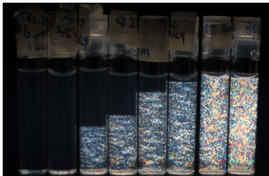
Figure 4. ZrP nanodisks suspensions with increasing concentrations from left to right observed between crossed polarizers. Volume fraction of the nanodisks from left to right: 0.38%, 0.44%, 0.50%, 0.53%, 0.56%, 0.63%, 0.75% and 1% respectively. The colorful portions indicate nematic ordering of disks. Due to gravity, nematic tactoids settle at the bottom. This picture is taken after 3 days of gravity sedimentation of nematic tactoids.
