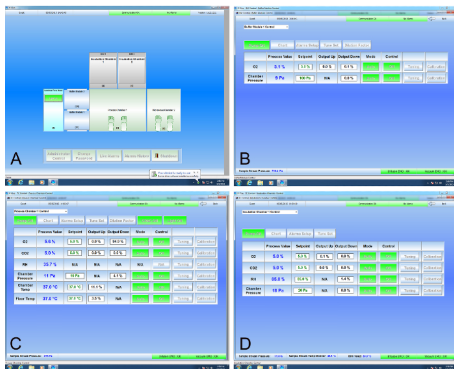
Figure 1. Graphical Interface for the Cell Production Facility. (A) The graphical representation of the CPF is the default screen and matches the CAD drawing shown in Figure 3. A click of the mouse over the Buffer Module 1 (2F in Figure 1) opens its control screen (B) where O 2 values are set to match the processing chamber (3 in Figure 3). Similarly, clicking on the Process Chamber or Incubator 1 brings up their respective control screens (C and D, respectively), where values may be changed or monitored as appropriate. Please click here to view a larger version of this figure.
