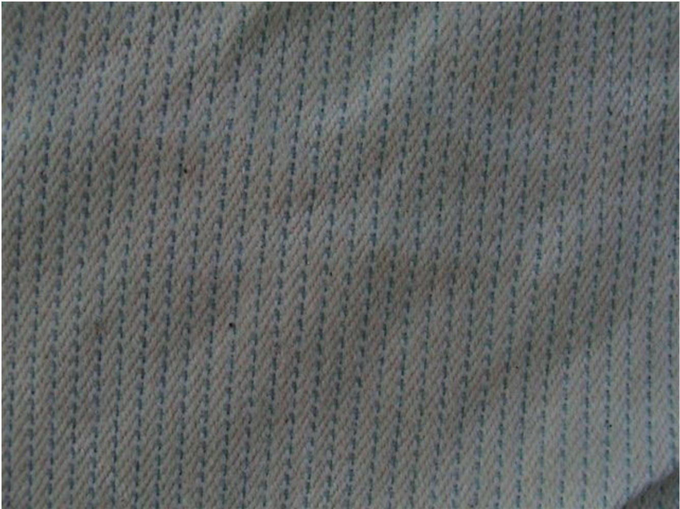
Figure 1 Close-up of tent material: canvas with delatemethrin-treated polyethelene thread woven through.
