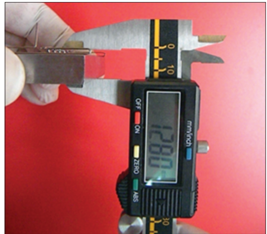
Figure 4: Vertical measurements with Vernier caliper
