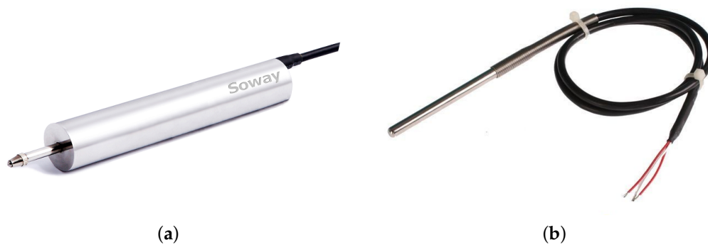
Figure 1. Sensors used for crack width change monitoring. (a) LVDT crackmeter; (b) PT100 temperature detector.
