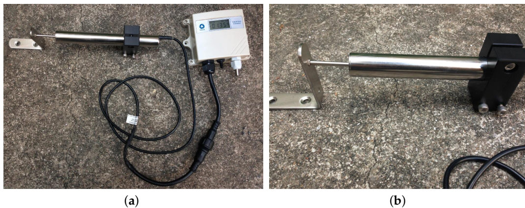
Figure 6. The installation of LVDT crackmeters. (a) The sensor node; (b) Installation details diagram.
