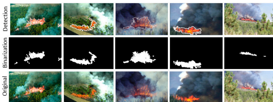
Figure 6. Examples for forest fire detections from aerial perspective.
