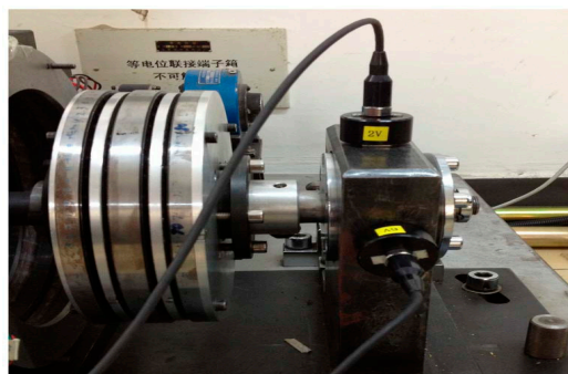
Figure 6. Experimental system and installation locations of the acceleration sensors.
