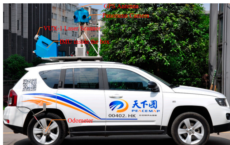
Figure 13. Mobile LiDAR system used for experiment dataset acquisition.
