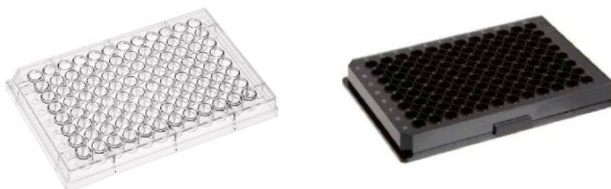
Figure 3: Examples of Layout for 96-well Plates. Top, table of the layout for loading a 3x drug plate for fluorometric plate reader, using three-fold concentrations of various neurotransmitters and peptides. Bottom, examples of clear plastic 96-well drug plate and black 96-well plate for seeding CNiFERS and measuring in plate reader. Please click here to view a larger version of this figure.
