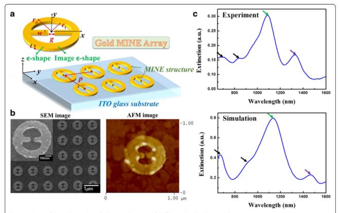
**Fig. 1** a Scheme of the MINE array design. **b** SEM and AFM images of the fabricated gold MINE array with t = 31 nm, g = 51 nm, w = 77 nm,  $r_i = 174$  nm,  $r_o = 304$  nm, and p = 1000 nm. The *inset* shows a magnified SEM image of a single gold MINE structure. **c** Extinction spectra of the MINE structure from the experiment and simulation
