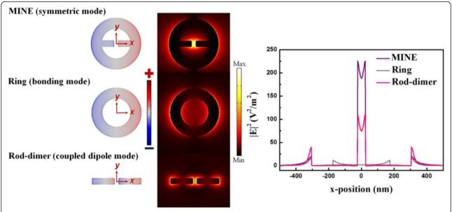
Fig. 3 Surface charge and field intensity distributions in the x-y plane and field intensity distributions along the x-direction of the MINE, nanoring, and nanorod dimer structures
