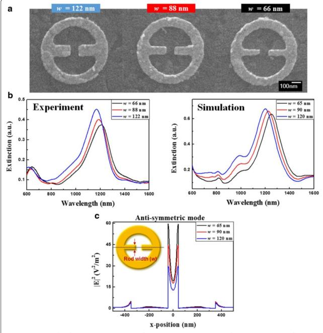
**Fig. 10 a** SEM images of the fabricated MINE structures with different rod widths. **b** Extinction spectra of the MINE structures with different rod widths for both experiment and simulation. **c** Field intensity distributions of the anti-symmetric modes of MINE structures along the *x*-direction with different rod widths
