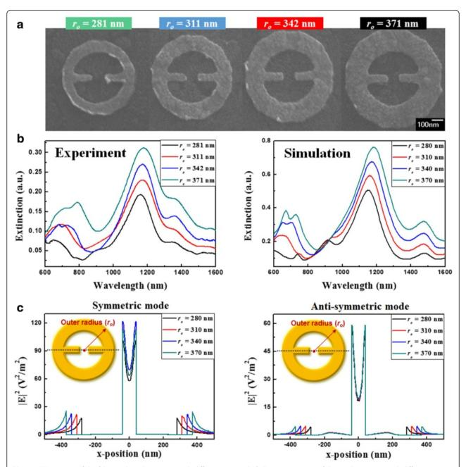
**Fig. 8 a** SEM images of the fabricated MINE structures with different outer radii. **b** Extinction spectra of the MINE structures with different outer radii for both experiment and simulation. **c** Field intensity distributions of the symmetric and anti-symmetric modes of MINE structures along the *x*-direction with different outer radii
