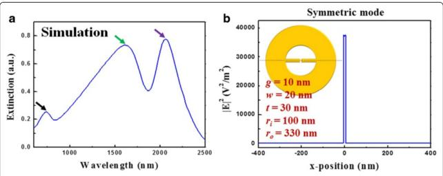
**Fig. 12 a** Extinction spectrum and **b** field intensity distribution of the symmetric mode along the *x*-direction of the MINE structure with g = 10 nm, w = 20 nm, t = 30 nm, t = 100 nm, and  $t_0 = 330 \text{ nm}$  on glass substrate
