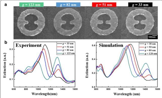
Fig. 4 a SEM images of the fabricated MINE structures with different gap distances. b Extinction spectra of the MINE structures with different gap distances for both experiment and simulation
