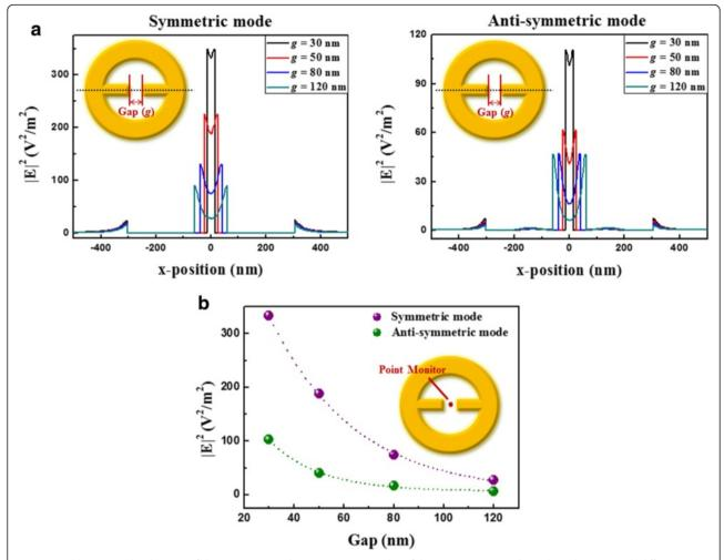
Fig. 6 a Field intensity distributions of the symmetric and anti-symmetric modes of the MINE structures along the x-direction with different gap distances. **b** Field intensities at the gap center of the MINE structure as a function of the gap distance
