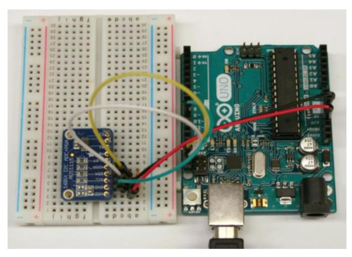
**Figure 1.** Photograph of the Arduino Uno, ADS1115 Analog-to-Digital Converter placed onto a circuit breadboard, and the wiring connections needed for the data acquisition device.
