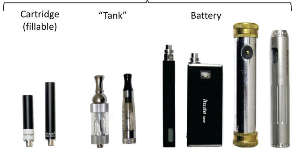
Figure 1. Examples of open and closed electronic cigarette systems.
