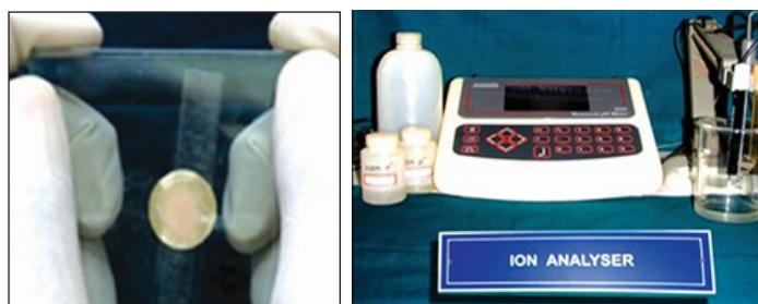
[Table/Fig-4]: Cement specimen preparation for fluoride estimation.
