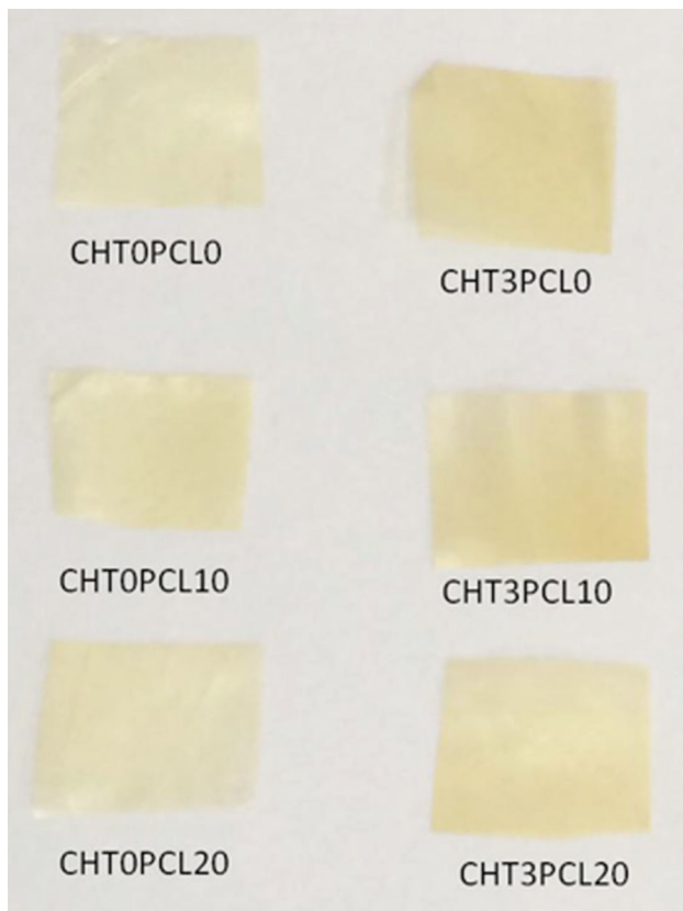
Fig. 1 Appearance of chitosan/PCL films prepared with different contents in PCL and \alpha -tocopherol. Codes as in Table 2
