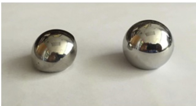
Figure 4. Photograph of a retrieved, misshapen, 28-mm, cobalt-chrome, modular femoral head (left) next to an unused head of the same size (right).
