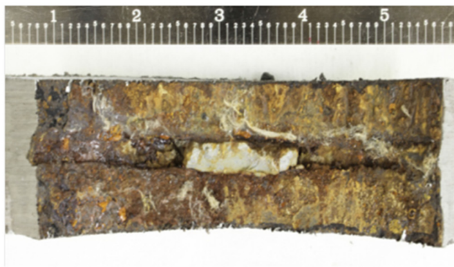
d) Optical micrograph of pitting at the leak site
