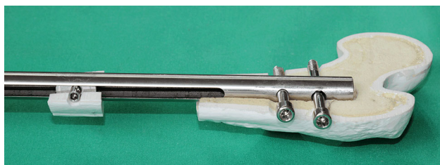
Fig. 5 CDS implanted into the femur with bone segment connected to the threaded rod via the spindle nut (lateral view)
