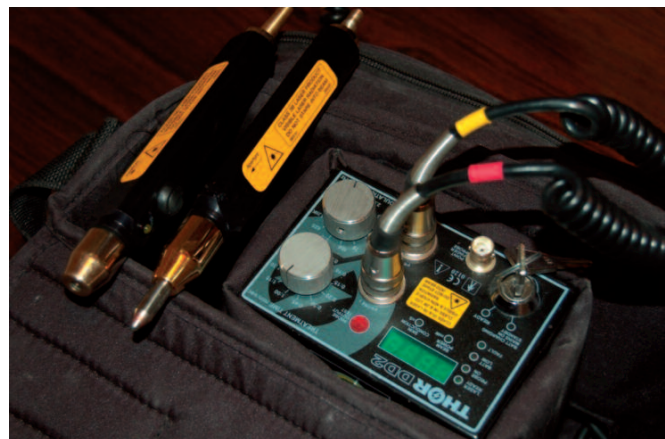
Fig. 2: The low power gallium-aluminum-arsenide (GaAlAs) and indium-gallium-aluminum-phosphide (InGaAlP) lasers used in this study
