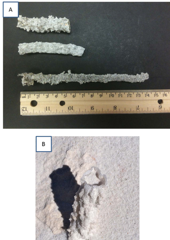
Figure 1. (A) Exemplary fulgurites collected from the field area. Surficial differences likely result from different initial physical conditions (e.g., percent water in sand). Color differences are apparently due difference between the thicknesses of the glass wall, which are 1.1 \pm 0.1 , 0.9 \pm 0.3 , and 1.6 \pm 0.3 mm from top to bottom (taken from 10 measurements, with 1 standard deviation given as the error). (B) Fulgurite found in situ . Diameter is about 1.2 cm.
