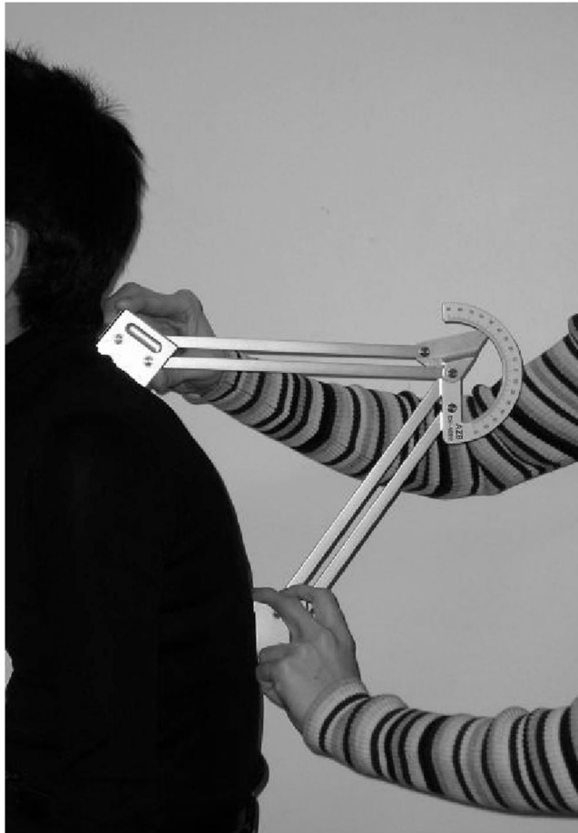
Figure 1. The Debrunner kyphometer is shown placed on a subject's spine.
