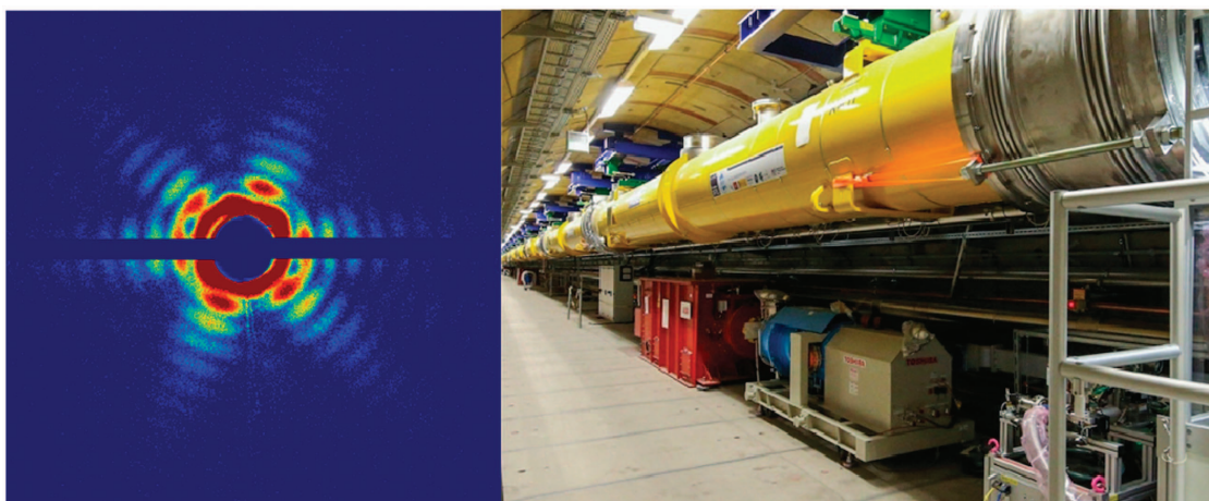
Figure 1. Diffraction patterns of a Mimivirus obtained at the LCLS 5 , and the newly built accelerator at the European XFEL (image on the right, courtesy of the European XFEL). The Collection of Data Descriptors contains many terabytes of images, but they will be quickly dwarfed by the data production rates of upcoming facilities such as the European XFEL and the upgraded LCLS II.
