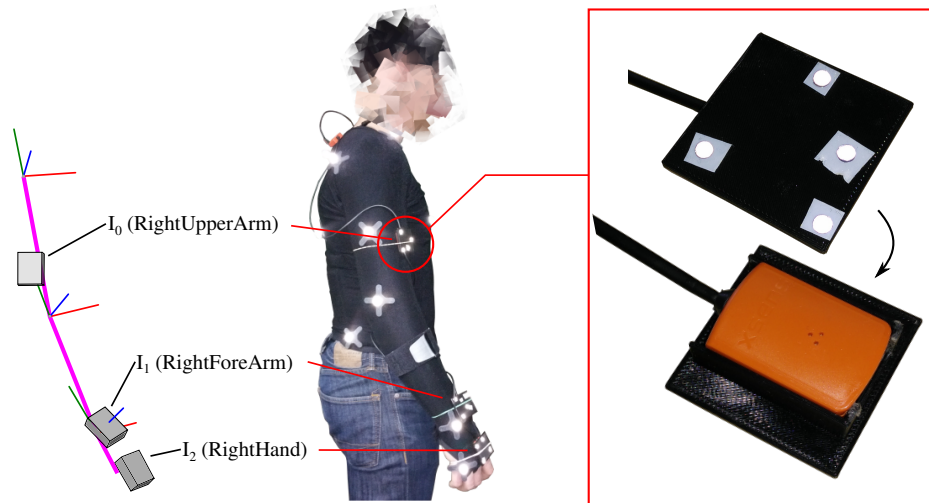
Figure 2. Capturing setup for the real data scenario. In the picture on the left, the segment coordinate systems are associated to the proximal ends of the segments. Note, the axes are orthogonal and only roughly aligned with the anatomical axes of rotation through the skeleton fitting of the optical system as described in Section 2.6.1. Precise alignment with the anatomical axes was not in the focus of this study. In the N-pose, for the right arm, the x -axes are chosen perpendicular to the frontal plane pointing anterior, the y -axes are perpendicular to the transverse plane pointing along the segments in the direction from the distal to the proximal ends and the z -axes are perpendicular to the sagittal plane pointing lateral. The picture also indicates the initial arm configuration for real-slow and real-fast .
