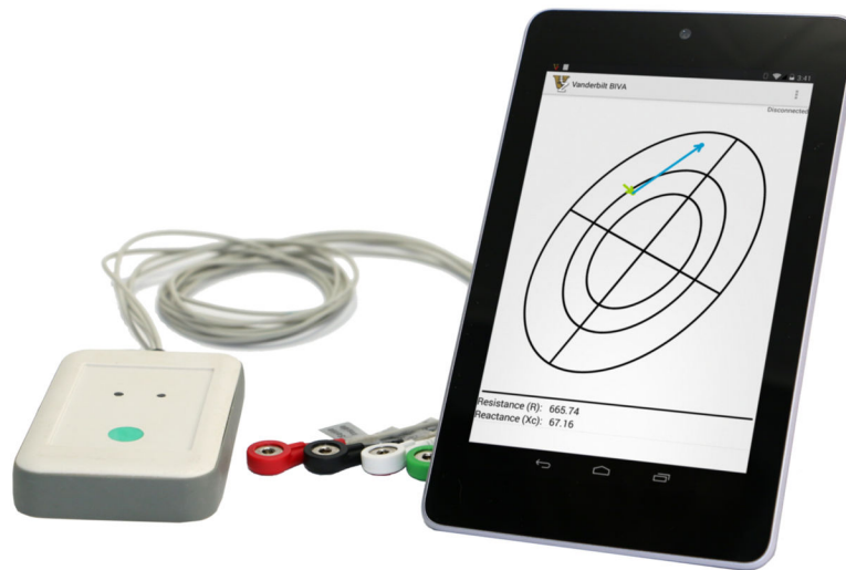
Figure 2. Wireless multi-frequency impedance spectrometer (left) used for bioelectrical impedance vector analysis (BIVA) in a rugged dust and water protected (IP 54) enclosure and snap on lead wires for easy and robust electrode attachment. Mobile application running on Nexus 7 tablet computer (right) that displays multiple BIVA measurements and allows for tracking of patient progress, patient management and data export.
