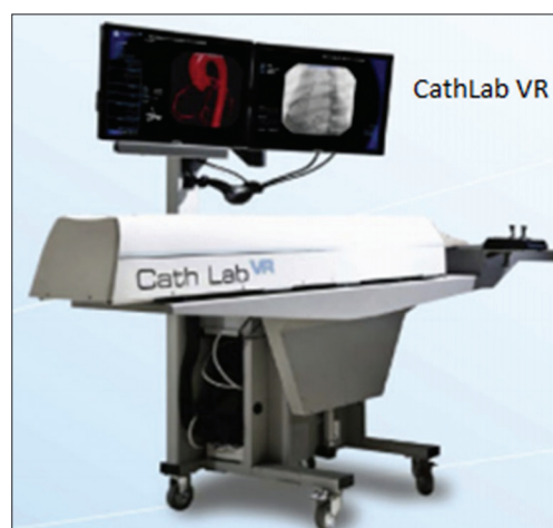
Figure 2: The Cath VR use for embolic protection devices, cardiac rhythm management, failed bioprosthetic valve management, transcatheter aortic valve simulation
