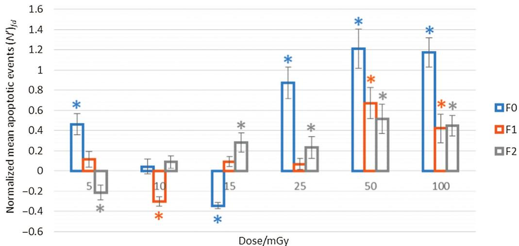
Fig. 1. Normalized mean apoptotic events ( $(N')_{fd}$ ) induced by 150 kV X-rays under the different filtration conditions of F0, F1 and F2, with respect to different X-ray doses. For each filtration condition, three sets of experiments were performed and the normalized data were pooled together. Cases with  $P < 0.05$  are asterisked and regarded as corresponding to statistically significant differences.
