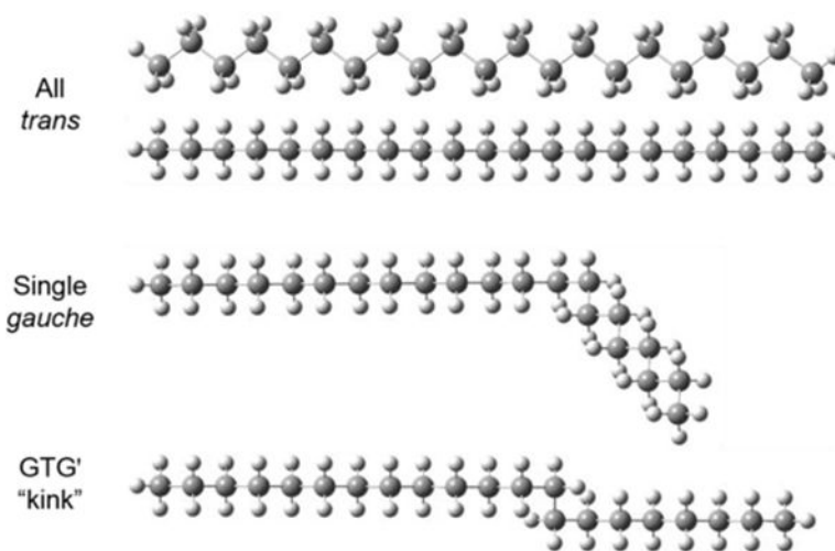
Figure 5. Structures of a C_{21} alkane in an all trans conformation and with either a single gauche bond or GTG' sequence.
