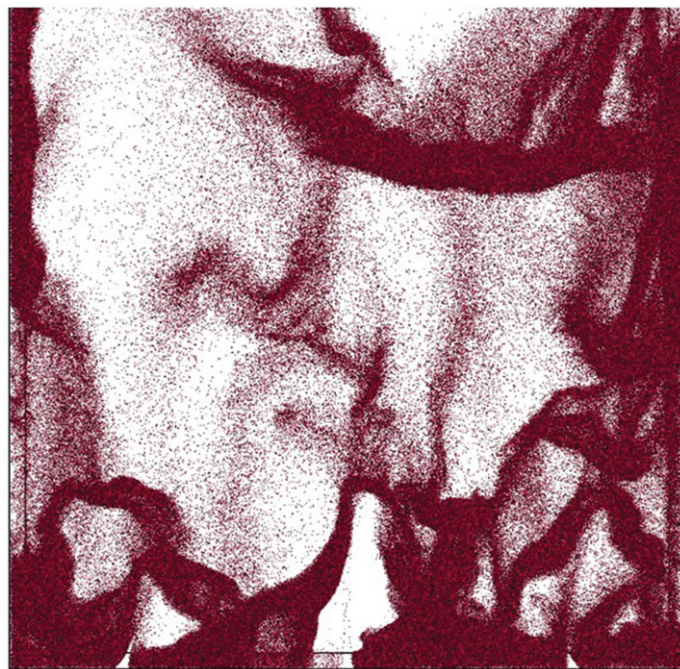
Figure 8. CFD-DEM of a fluid bed process involving 25 million particles. The fine structure of particle clusters (streamers) can be observed. For details regarding the simulation setup refer to Jajcevic et al. 155
