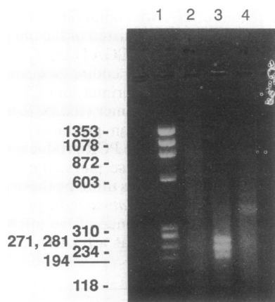
FIG. 2. Agarose gel electrophoresis of the products of PCR amplification of cDNA. The PCR was carried out with cDNA prepared from poly(A) RNA isolated from E. coli SK5726 after a shift to 44°C (see Fig. 1), by using one general primer (Fig. 3, PCR primer 2) and one gene-specific primer. Samples of the reaction products were electrophoresed in 3% agarose gels and stained with ethidium bromide. Lanes: 1, Hae III digest of bacteriophage ΦX174 DNA; 2, product obtained with a lacA -specific primer (5'-ACGTCTG-GATCGGAAGTCATGTGGT-3'); 3, products obtained with a lpp -specific primer (5'-AGCAACGCTAAAATCGATCAGC-3'; Fig. 3, PCR primer 1); 4, products obtained with a trxA -specific primer (5'-GACACGGATGTACTCAAAGCGGACG-3').
