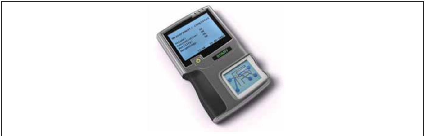
Figure 1 An artistic impression of the fertility chip. It consists of a handheld system, microfluidic chip and software.
