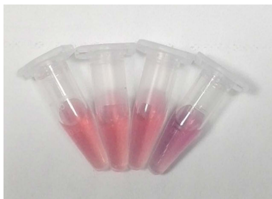
Figure 3. Photograph of color changes caused by adding HBeAg to aptamer-linked AuNPs. From left to right: aptamer-linked AuNPs + 0.09 M NaCl; aptamer-linked AuNPs + 50 nM parynzyme + 0.09 M NaCl; aptamer-linked AuNPs + 50 nM HBeAg + 0.09 M NaCl; aptamer-linked AuNPs + 50 nM HBeAg + 0.09 M NaCl.
