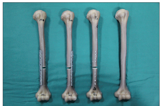
Figure 1: Anatomical reduction was observed in all specimens after fixation of the fractures with plates and screws.
