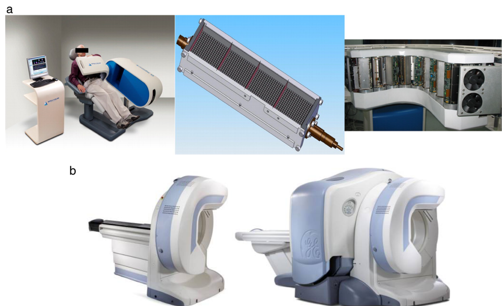
Fig. 1 CZT (cadmium-zinc-telluride)-based gamma cameras. a D-SPECT (Spectrum Dynamics Medical): overview, one of nine detectors, and a gantry with nine detectors from left to right. (This figure was originally published by Gambhir et al. [7]. Copyright the Society of Nuclear Medicine and Molecular Imaging). b Discovery 530c (GE Healthcare) ( left ), NM/CT570c (GE Healthcare) ( right ). (This figure was originally published by Bocher et al. [73] under the terms of the Creative Commons Attribution Noncommercial License. No change was made)
