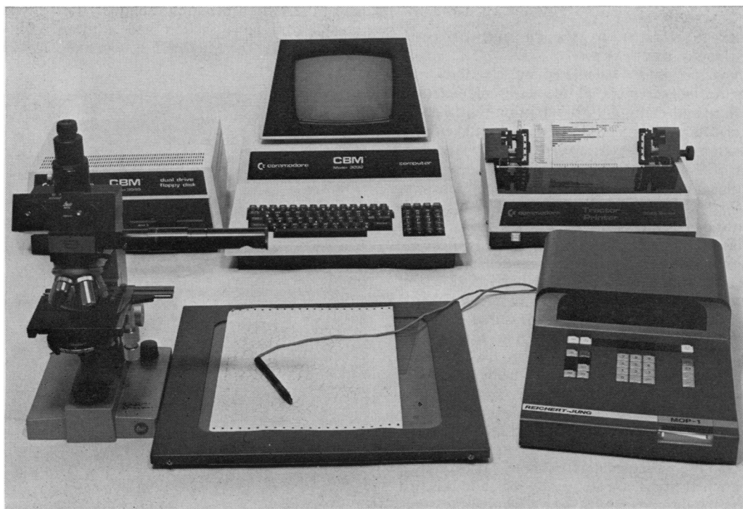
Fig. 1 Microscope and microprocessor system for measuring cell areas. Front, left to right, microscope with drawing tube side arm, MOP drawing tablet, MOP microprocessor. Back row left to right, disk storage unit, PET computer, printer.
