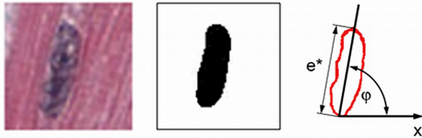
Fig 4. Fibre orientation based on the shape of a nucleus. The left image shows a small detail of a sample image visualizing a nucleus, the image in the middle represents the segmented nucleus as a binary image. The graph on the right depicts the scheme of determination of the angle of orientation. e^* denotes the longitudinal axis of the nucleus cutting contour in the xy - image plane. The angle \varphi represents the in-plane angle of the nucleus with respect to the x -axis. Image size = 20 \mu\text{m} \times 20 \mu\text{m} .
