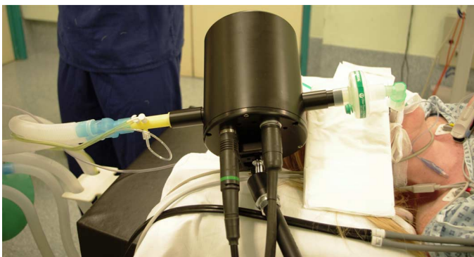
Fig. 1. MFS in use during surgery. MFS measurement head incorporated in a closed-loop anesthetic delivery system. A 5-m-long pair of cables connects the measurement head to the control unit located away from the operating table.
