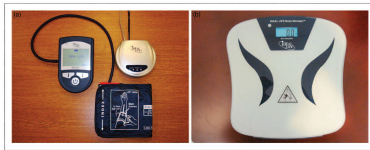
Figure 1. Telehealth system – patient equipment (a) Blood pressure measuring unit (left) and wireless transmission unit (top right); (b) Bodyweight scale.
