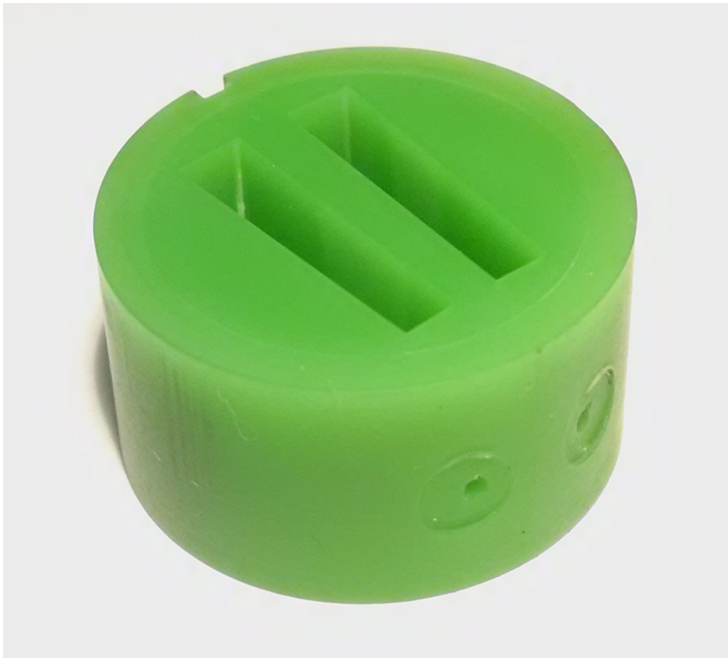
Fig 1. Picture of a 12 mm pathlength centerpiece printed of ABS-like resin MicroFine Green. Sedimentation velocity data of BSA at 50,000 rpm collected with this centerpiece installed into a standard cell assembly without gaskets are shown in Fig 3B .
