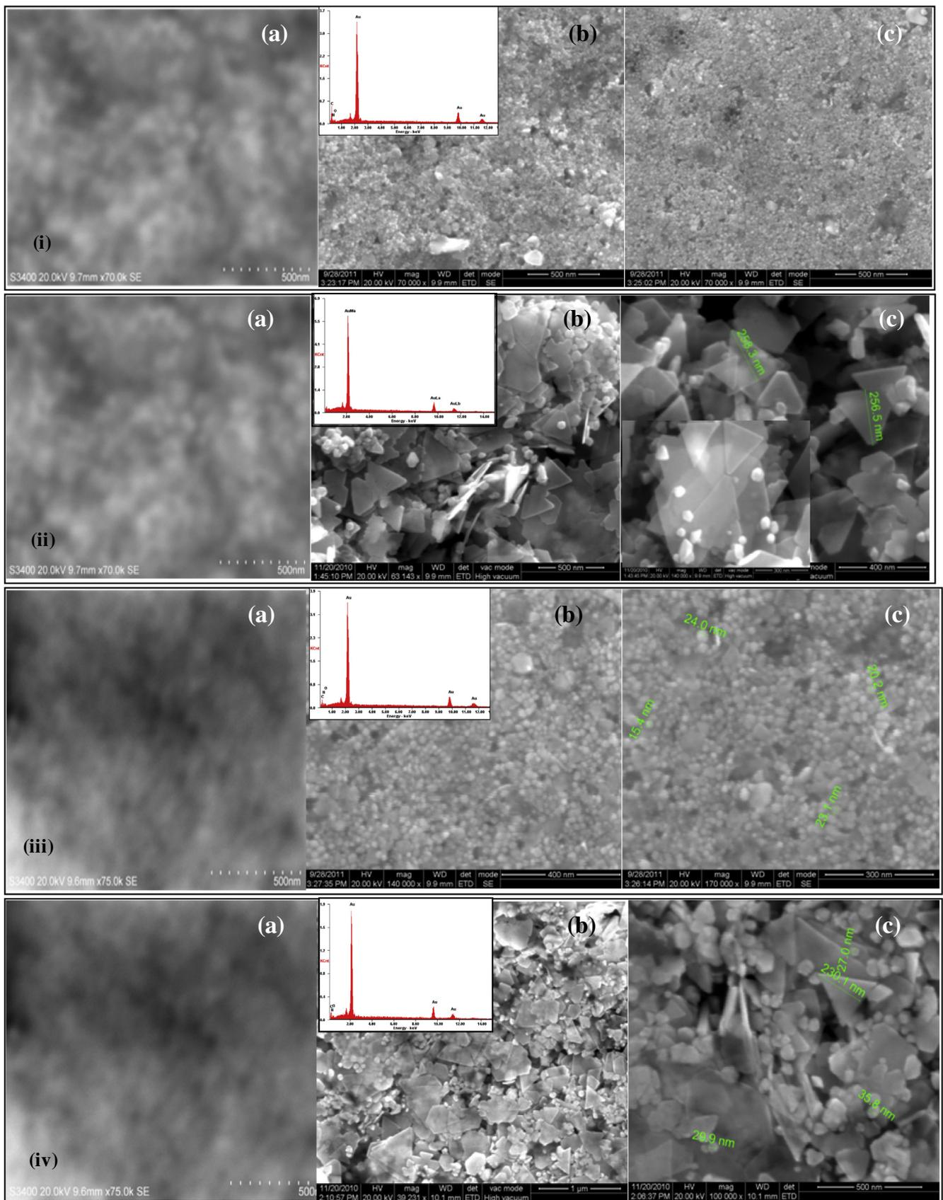
**Fig. 3** A composite visual of (a) scanning electron micrograph; (b and c) high resolution scanning electron micrographs (inset is the EDX spectrum) of gold nanoparticles formed with the extracts of the aerial parts (i and ii), and submerged parts (iii and iv) of pistia.
