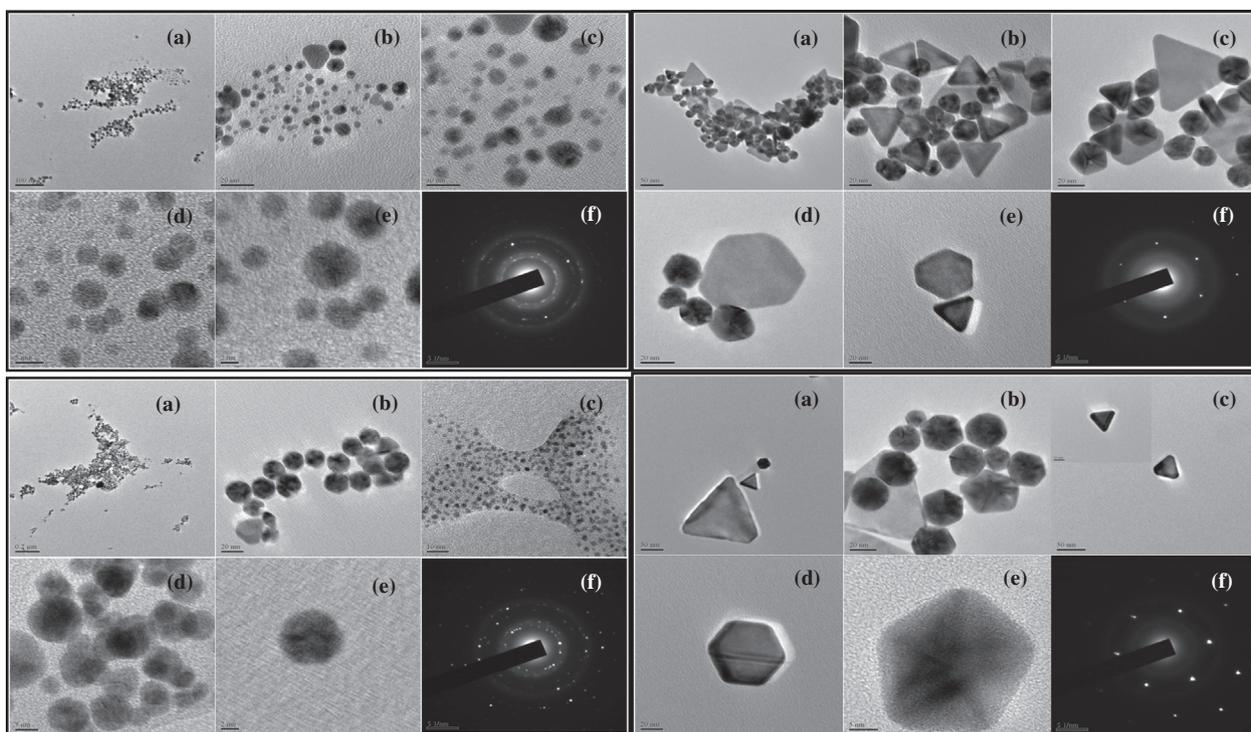
**Fig. 4** A composite visual of transmission electron micrographs (a–e) showing hexagonal, pentagonal and triangular particles of gold nanoparticles formed with the extracts of the aerial parts (i and ii), and submerged parts (iii and iv) of pistia.
