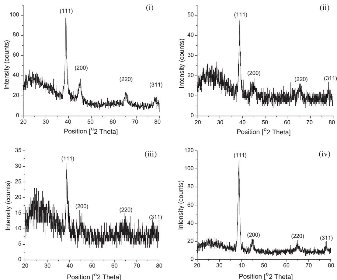
**Fig. 5** X-ray diffraction spectrum of gold nanoparticles formed with the extracts of the aerial parts (i and ii), and submerged parts (iii and iv) of pistia.
