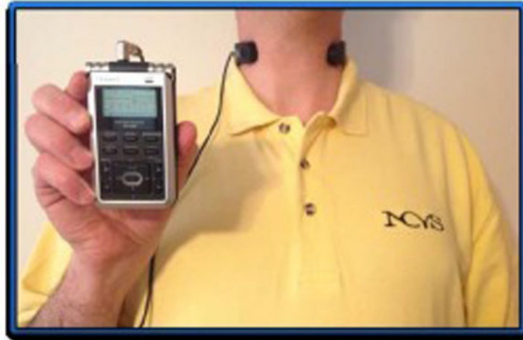
Figure 2. VoxLog™ collar worn around the neck and attached to a Roland R-05 Digital Recorder.
