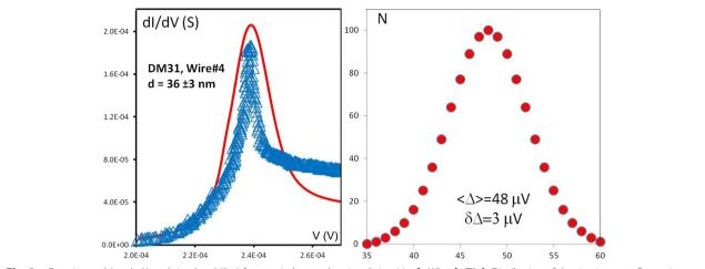
**Fig. 3 a** Experimental (*symbols*) and simulated (*line*) for a typical gap-edge singularity  $eV = \Delta_1(AI) + \Delta_2(TI)$ . **b** Distribution of the titanium gap fluctuations used in fitting data from panel **a**:  $|\tilde{\Delta}_2| = 48 \,\mu\text{eV}$ ,  $\delta|\Delta_2| = 3 \,\mu\text{eV}$
