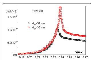
**Fig. 2** First derivative dV/dl characteristic: blow-up of the singularity at eV =  $\Delta_1(Al) + \Delta_2(Ti)$  of two  $S_1 I S_2$  junctions with two titanium electrodes of different effective diameters  $d_{\rm eff}$  equal to 31 and 36 nm (indicated in the *inset*). One can clearly see that for the thinnest titanium electrode, the absolute value of the mean gap  $\left|\tilde{\Delta}_2\right|$  is smaller and the broadening  $\delta |\Delta_2|/\left|\tilde{\Delta}_2\right|$  is larger
