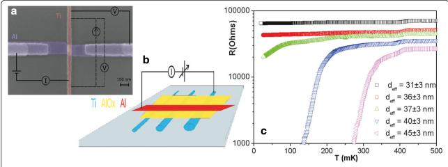
**Fig. 1 a** SEM image of a typical  $Al-AlO_x$ -Ti tunnel junction with schematic of the electric circuit. **b** Schematic of the nanostructure layout. **c** R(T) dependencies of titanium nanowires with various effective diameters  $d_{\text{eff}}$
