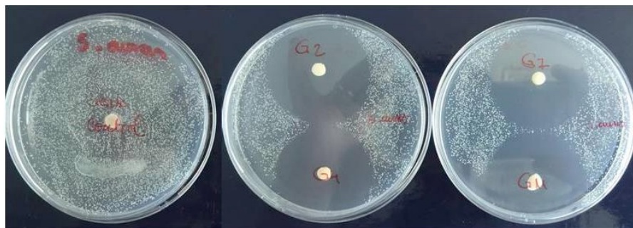
Figure 1. Antimicrobial efficacy test for Staphylococcus aureus showing inhibition zone around gentamicin coated FRC discs.
