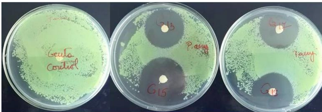
Figure 2. Antimicrobial efficacy test for Pseudomonas aeruginosa showing inhibition zone around gentamicin coated FRC discs.
