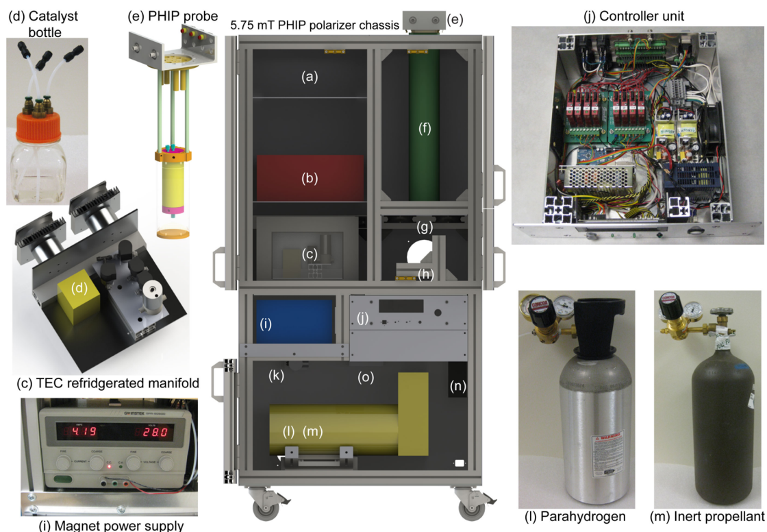
Figure 1. Schematic of the PHIP hyperpolarizer. The system consists of the following key elements: (a) a device frame, (b) NMR spectrometer and RF amplifier(s), (c) thermoelectric cooled (TEC) manifold, (d) catalyst/precursor containing bottle, (e) PHIP probe, (f) B_0 magnet, (g) B_0 magnet/RF probe cooling fans, (h) interface to HyperBridge, (i) B_0 magnet power supply unit (PSU), (j) controller unit, (k) solenoid valves, (l) para - H_2 tank, (m) propellant inert gas tank, (n) power distribution unit, and (o) step-down pressure regulator. The overall hyperpolarizer dimensions are \sim 68 in. (height) by \sim 21 in. (depth) by 33 in. (width). See additional details in the text and Supporting Information .
