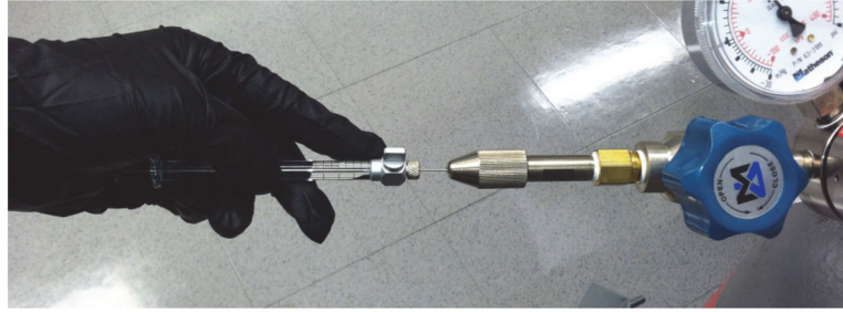
Figure 3. Methane gas tank fitted with a septa
