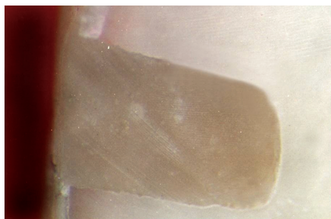
Fig. 7: Score 1: Dye penetration along occlusal wall but less than ½ way to axial wall
