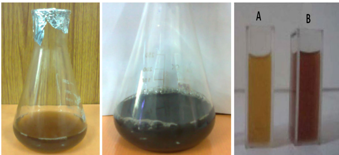
Fig. 1 Conical flask with silver nitrate ( Ag-100 ppm) before (1) and after (2) exposure to A. marina showing AgNO_3 a silver nanoparticles after 6 h and b 72 h
